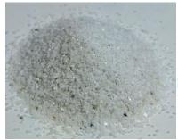
Calcite (calcium carbonate) is slow to react, requires a lot of contact time with the water and corrects only up to a pH of about 7.0.
